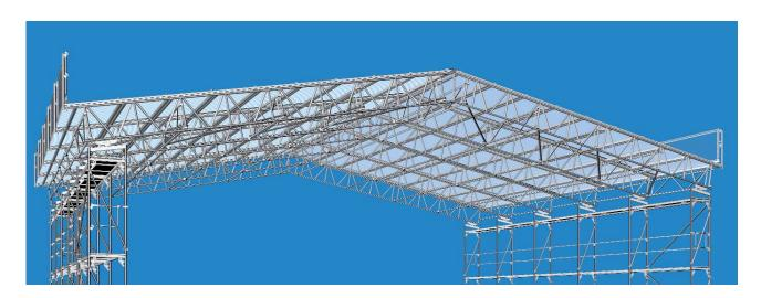
The lightweight cassette roof (LWCR) is a very light roof with a roof covering of aluminium/PVC roof cassettes that can be erected on non-system lattice girders. With a few extra parts, sturdy yet lightweight roofing can be provided for a wide range of applications.
